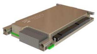
Mercury Systems' new TRRUST-Stor™ VPX RT spacequalified radiation-tolerant secure solid-state drives (SSD) featuring BuiltSECURE™ technology.
