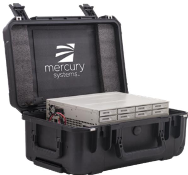
Mercury's RESmini XR6 server features the latest Intel® Xeon® Scalable (Skylake) processors, comes bundled with a new FAA-compliant power case and can operate independently for two hours without a power source.
