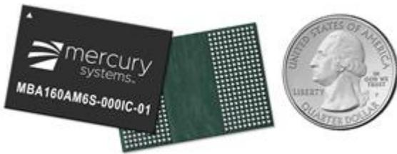
Mercury's TRRUST-Stor® Ball-Grid Array Solid State Drive (SSD)
