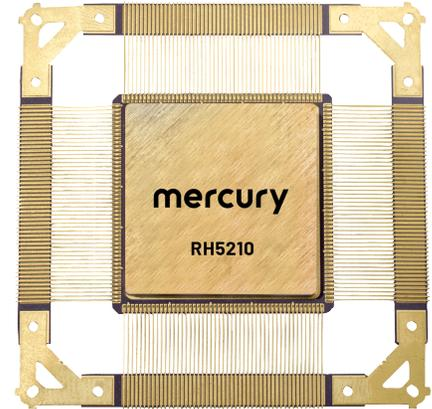
Mercury Systems' new RH5210 power module provides a drop-in SWaP-optimized power solution for many radiation-sensitive applications and platforms.
