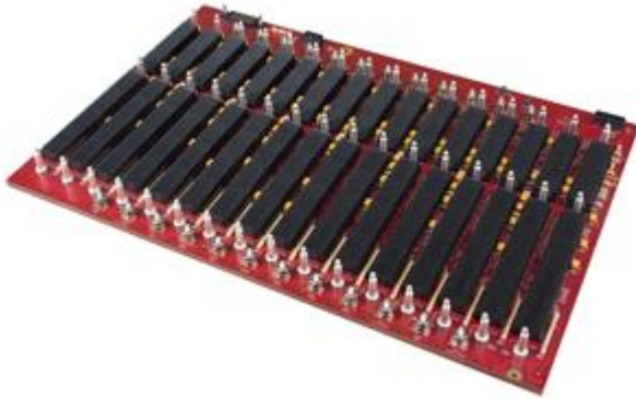
Mercury Systems' next-generation 100Gbps OpenVPX backplane
