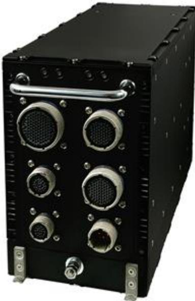
Mercury's ROCK-2 Avionics Platform, ideal for a wide range of mission computing applications, is available in all levels of flight safety design assurance levels from DAL-E to the highest, DAL-A.
