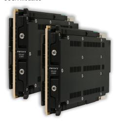
Mercury's new Model 5585 and Model 5586 SOSA aligned Xilinx Virtex UltraScale+™ FPGA 3U VPX modules are the first open architecture 3U products on the market to feature high-bandwidth memory, offering a 20x increase in memory bandwidth over traditional DDR4 memory.
